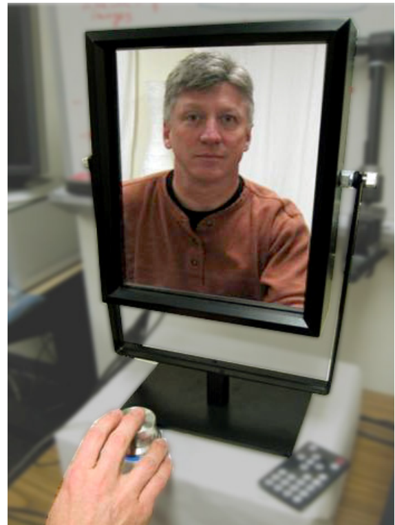
Figure 2. Countertop Responsive Mirror (P2). Mirror component consists of camera behind half-silvered mirror.
